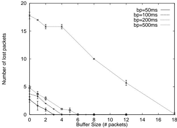
Figure 7: This graph shows the number of packets lost due to a handoff, from a stream of UDP packets that mimics an audio stream.
