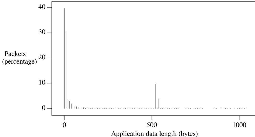
Figure 4 - Histogram of TCP application data lengths
