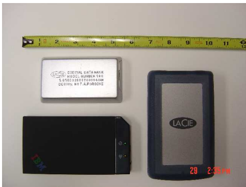
Figure 2: A sample of USB 2.0 portable disks used as SoulPads . Clockwise from upper left: LaCie 40GB DataBank, LaCie 60GB PocketDrive, and IBM 40GB Portable Hard Drive.
